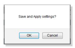
Selecting OK to the above question will activate most Quick Config settings. Some parameters, like the IP address of the Vega, will however require the Vega to be re-booted. If a reboot is required the Vega will ask whether this should occur immediately or whether you wish to do it manually later. If later is selected, the reboot button on the left hand side menu will be left RED to indicate that a reboot is still required to activate certain new parameters.
