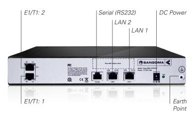
Both the Vega 100G and Vega 200G have both E1/T1 ports activated. The capacity of simultaneous VoIP calls that can be made is as follows:
